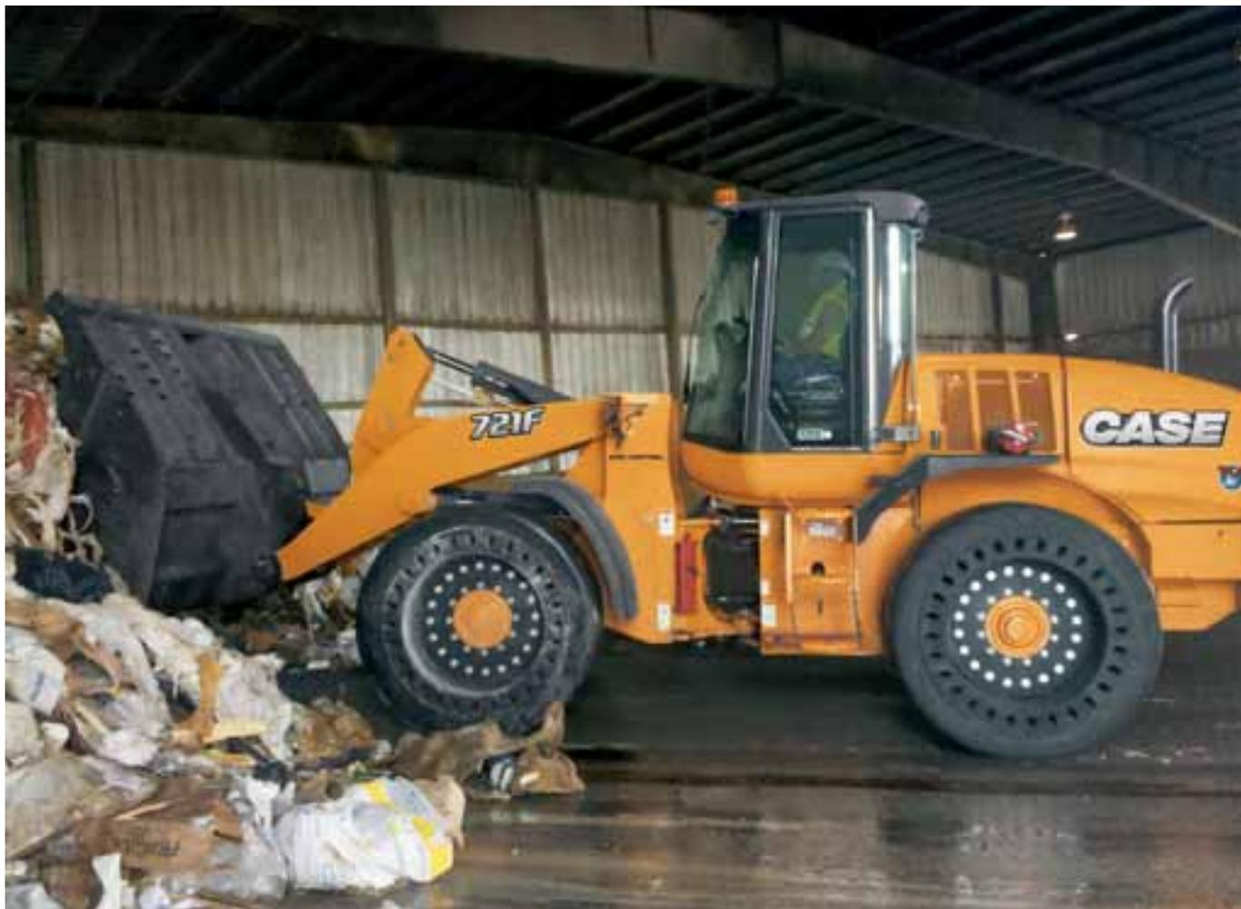
With L5 tyres, needed for work in very abrasive environments, we recommend heavy-duty axles. Solid tires can be retrofitted
