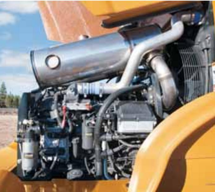
The layout of the components under the hood is optimized and results in easier maintenance.
