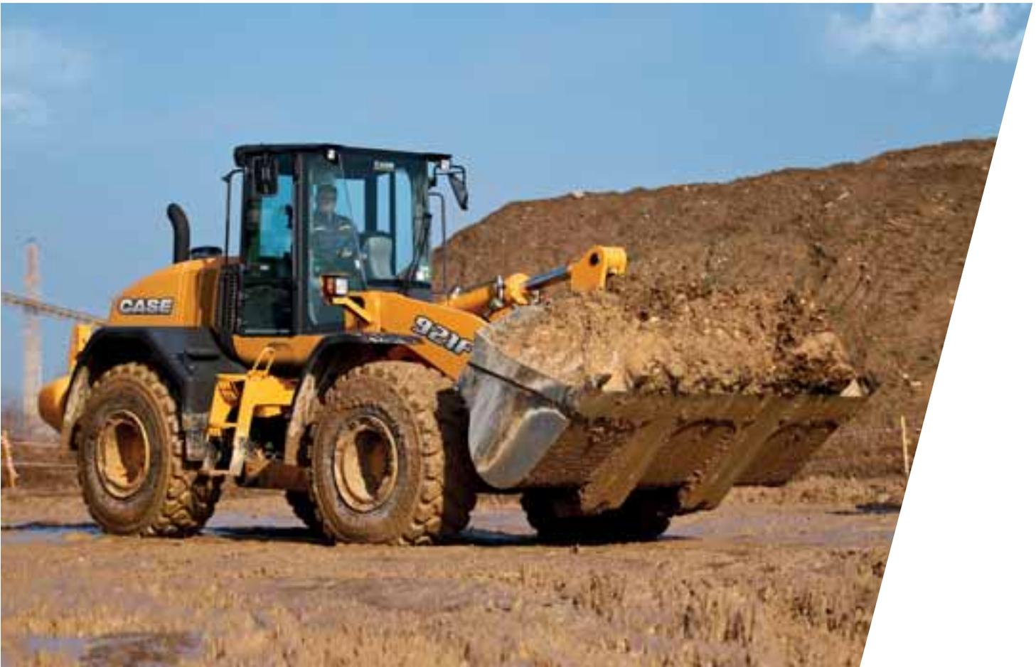
With L5 tyres, needed for work in very abrasive environments, we recommend heavy-duty axles. Solid tires can be retrofitted
